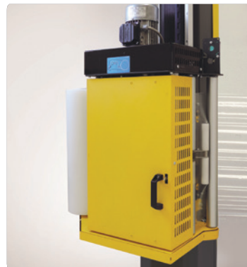
LP - Powered pre-stretch 240% (200% - kit available as option)
